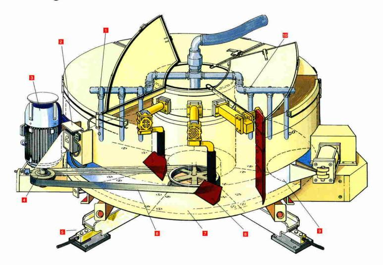
Intensive **Batch Mixing** With Uniform Wetting Produces a Homogenous. Stabilized Mix
