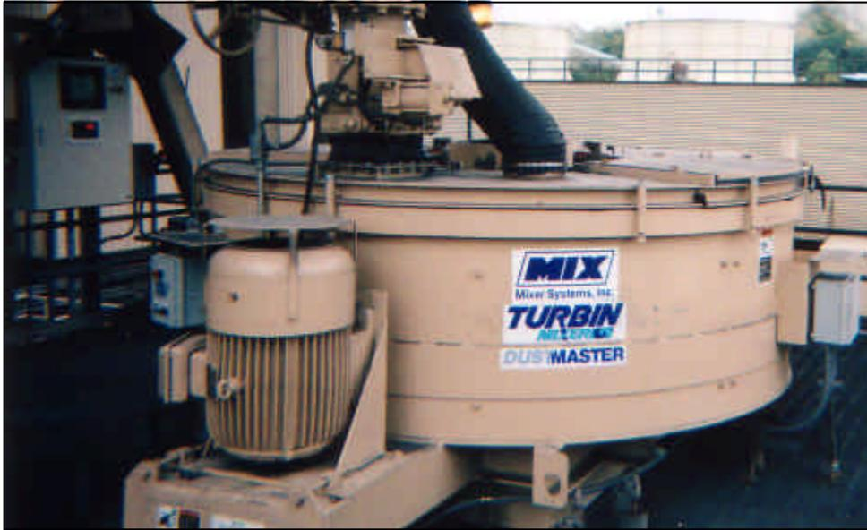
Mixer Systems' 60 tph DustMASTER Series II system for processing fly ash.
