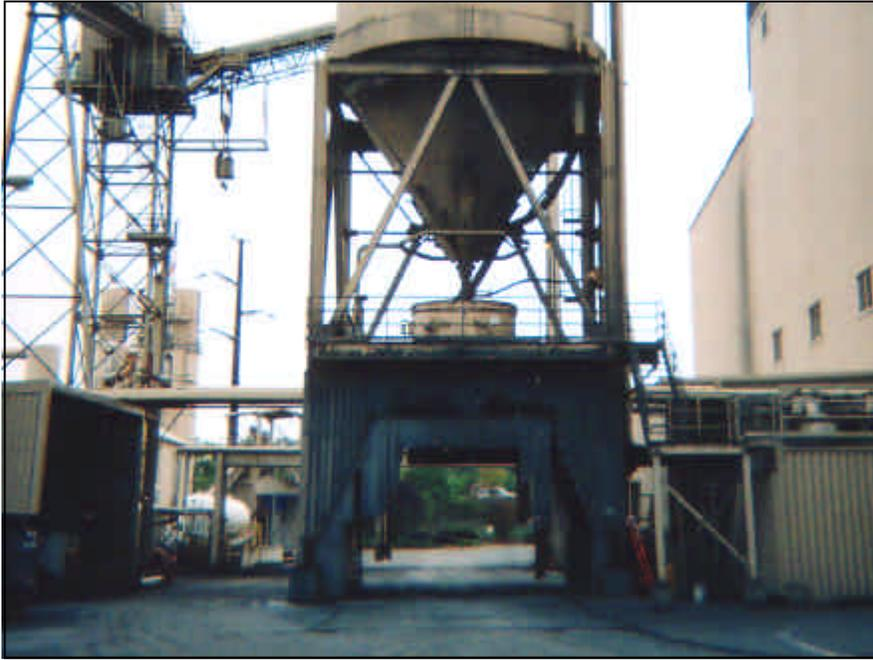
Stabilizing cupola and general bag house dust at this foundry is a 60 tph DustMASTER Series I system.
