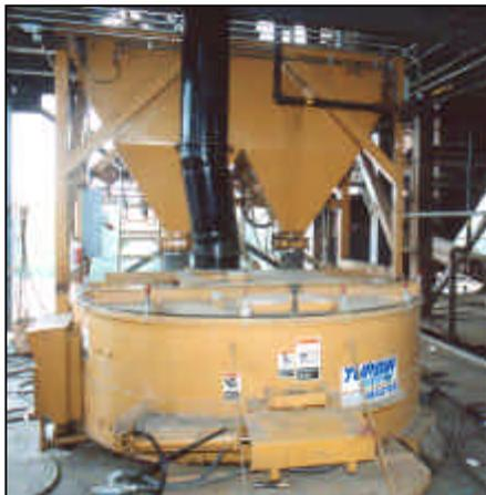
The 60 tph DustMASTER Series I is installed with weigh hoppers and the Mixer venting system.
