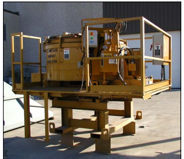
The 20 TPH DustMASTER size test mixer with stand.
