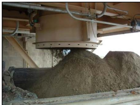
DustMASTER 40 TPH Series II mixer discharging conditioned flyash into truck.
