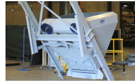
Bottom-dump bucket allows for easy, direct mixer feed
