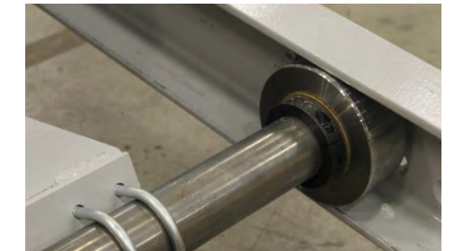
Machined track wheels with bearings roll smoothly
