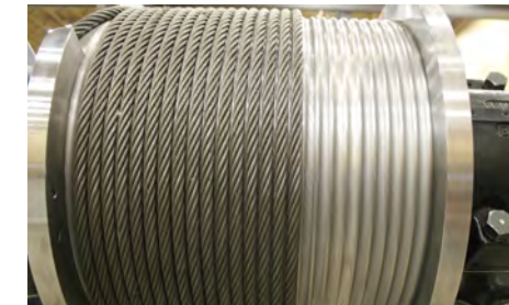
Machined cable drum prevents cable climbing and flattening
